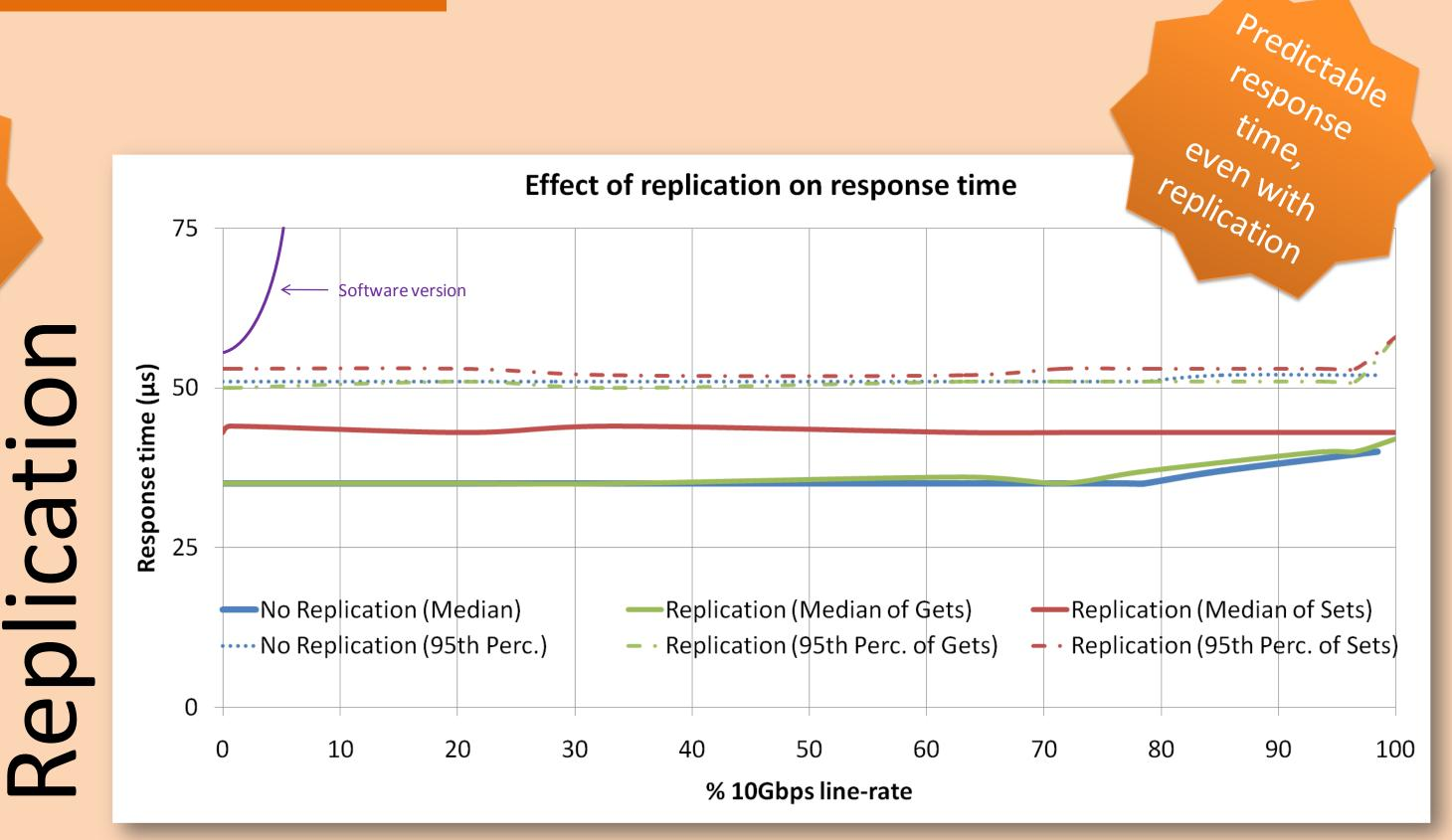
We measured the response time using memaslap, over UDP protocol. Key size =16B, Value size=512B, 10% Write workload. No replication: 1 FPGA. Replication: 2 FPGAs connected in ring. Software: Memcached 1.4 on dual socket Xeon E5-2609.
